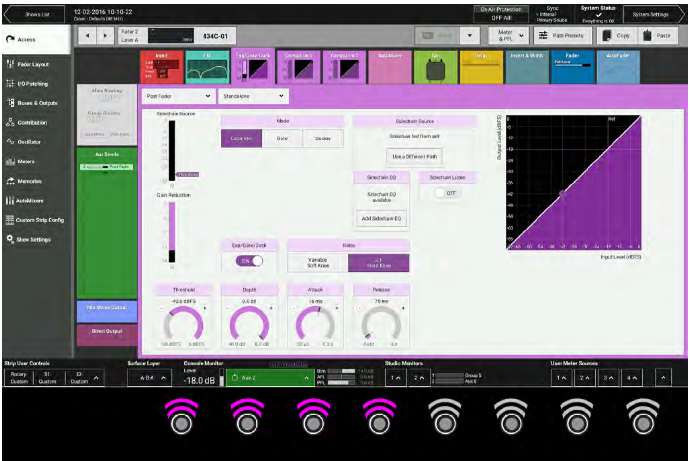
FIGURE 1 - CONTEXT CONTROLS—ACCESS MODE—EXPANDER/GATE/DUCKER
