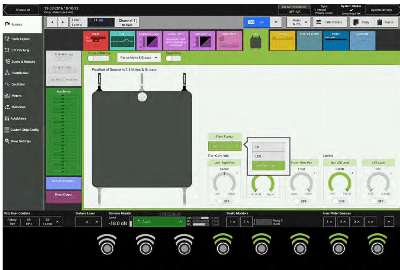
FIGURE 1 - CONTEXT CONTROLS—ACCESS MODE—MAINS & GROUPS PANNING
