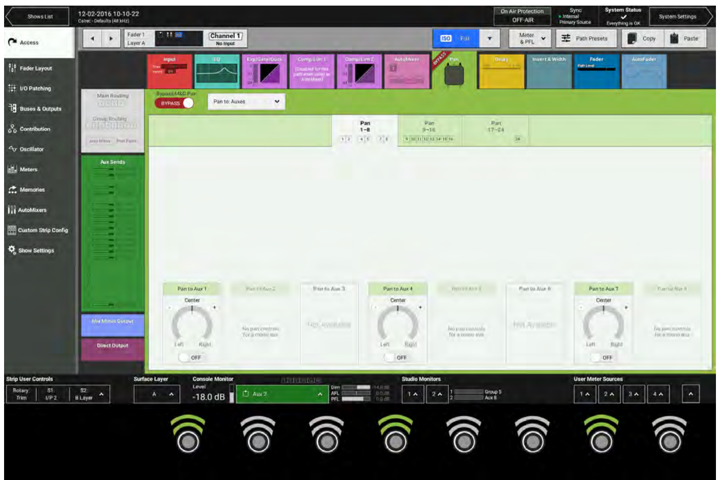
FIGURE 2 - PAN TO AUX CONTROLS
