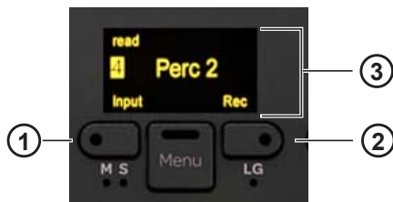
Input (1) and Record (2) switches, OLED (3)
