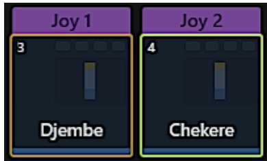
Figure 88. Joystick 1 (left) assigned but not stored in a Layout, and Joystick 2 (right) assigned and enabled to be stored (green highlight)
