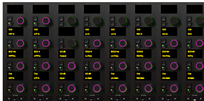
Figure 108. Attention Expand Knob Zone with expanded EQ3 7-band (plug-in bypass via column 8 Back switch)
