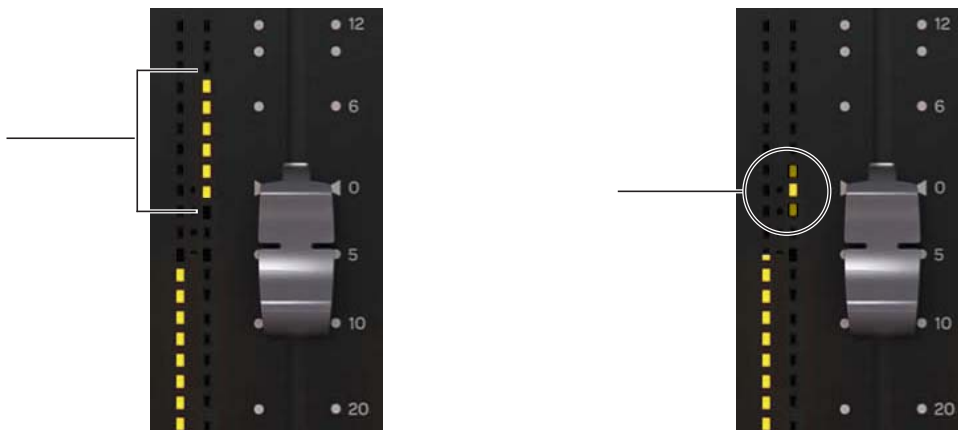
Figure 80. Automation Trim meter when editing Trim data (left) and Write indication (right) in strip meters
