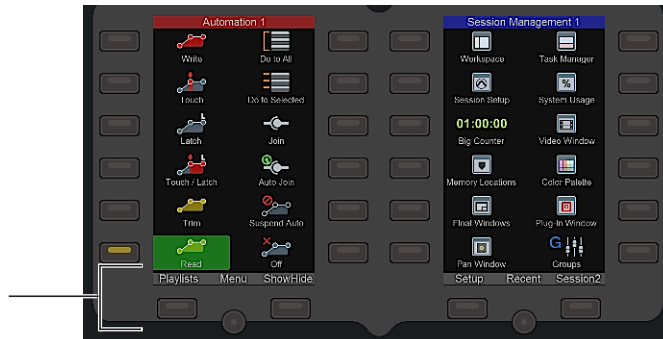
Navigation switches along the bottom of the left Soft Key bank on the Master Module (default Pro Tools appset)
