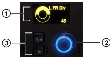
OLED (1), knob (2), and In and Sel switches (3) for the knob
