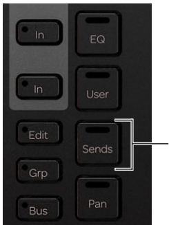
Sends switch on the Process Module
